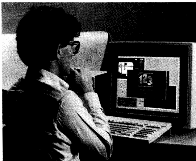
HP's new Series 300 DOS Coprocessor bridges the gap between UNIX and MS-DOS operating systems, creating a dual-purpose computer.
